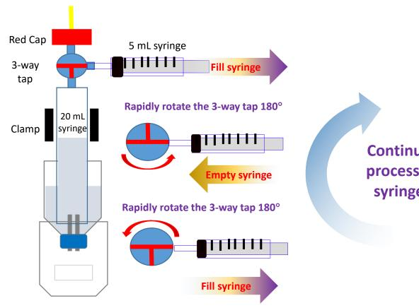
Continue this syringing process until the 20 mL syringe is completely filled
