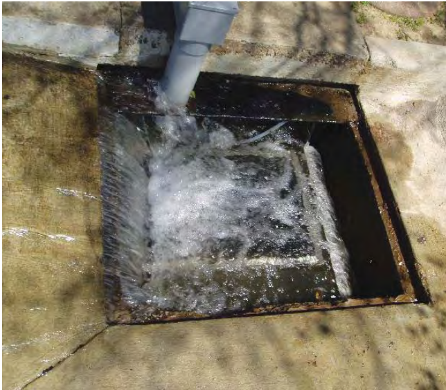
Exhibit 2.15 Hydro's Up-Flo filter during field pilot testing and verification
