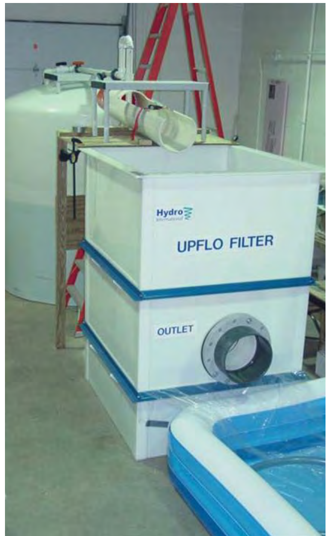
Exhibit 2.37 Hydro International's Up-Flo system during on-site pilot testing and ETV verification by Penn State University
