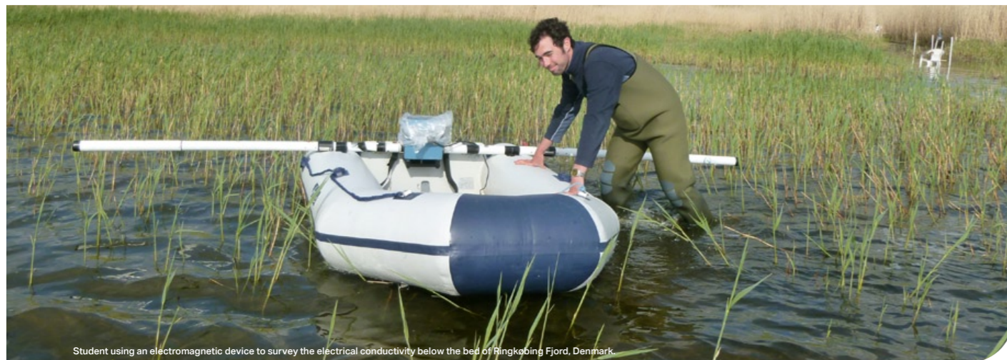
Student using an electromagnetic device to survey the electrical conductivity below the bed of Ringkøbing Fjord, Denmark.
