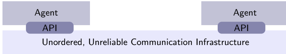
Fig. 1: MAS where agents communicate via a bare-bones infrastructure that guarantees neither message ordering nor delivery. The API represents programming abstractions offered by the infrastructure.
