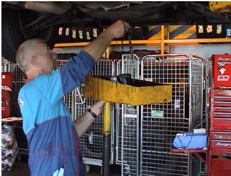
Figure 5: Draining the oil
