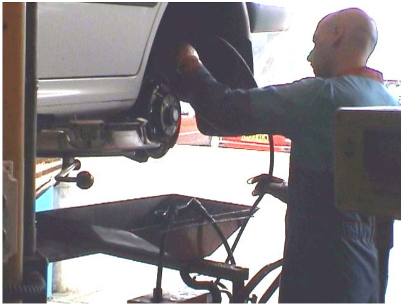
Figure 11: Special brake cleaning system with water-based, recycled degreaser
