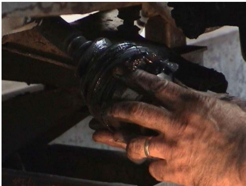
Figure 6: Applying grease to a constant-velocity joint
