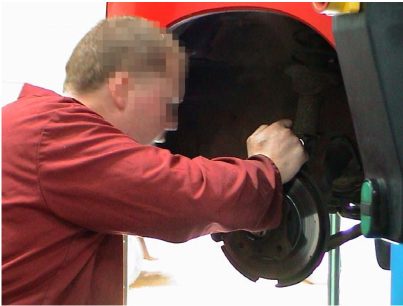
Figure 7: Blowing dust from a brake assembly
