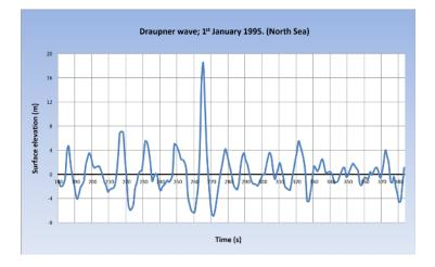
Laser readings, 1 January 1995. Wave 25.6m, crest 18.5m (Equinor)
