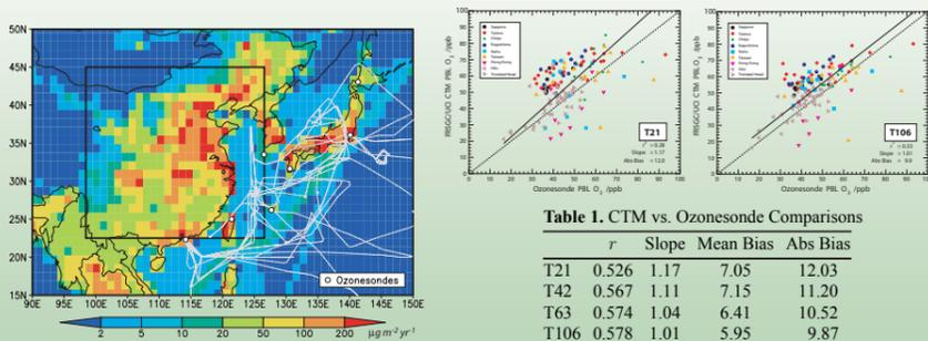
Surface NO<sub>x</sub> emissions over East Asia in March 2001 at T106 resolution. Ozone sonde launch sites and NASA DC-8 and P-3B aircraft flight tracks during the TRACE-P campaign are indicated; the region used for diagnostics is highlighted.
