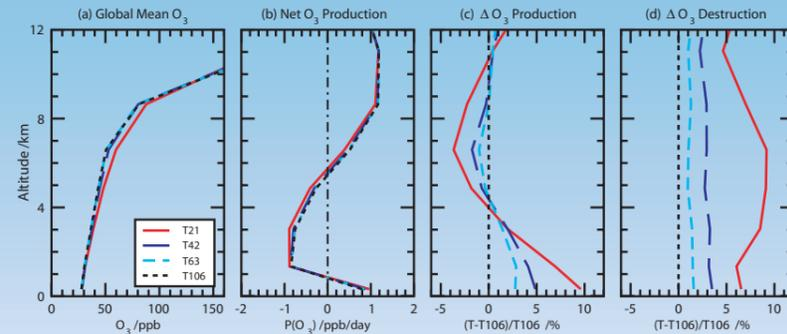
Impacts of resolution on the global O<sub>3</sub> budget for March/April 2001 showing (a) the mean O<sub>3</sub> profile, (b) the net chemical tendency, (c) the change in gross production relative to the T106 simulation, and (d) the change in gross destruction relative to T106.
