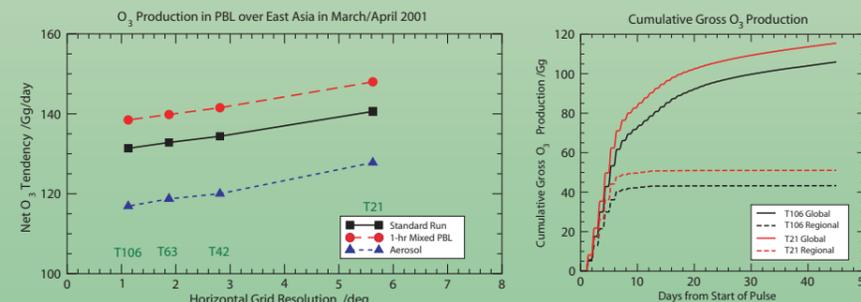
Net O<sub>3</sub> production over East Asia in springtime is 7-8% less at T106 than at T21, largely due to reduced distribution of emitted precursors. Alternative model formulations: (1) more rapid PBL mixing (greater mixing, higher O<sub>3</sub> production) and (2) climatological aerosol loading (reduced photolysis, slower production) both show similar impacts due to resolution.
