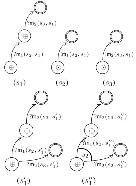
**Figure 3: Substituting  $s_1$  by  $s'_1$  causes a race condition, while substituting it with  $s''_1$  does not; the arc in  $s''_1$  expresses the fact that both alternatives are expected from  $s_2$ .**
