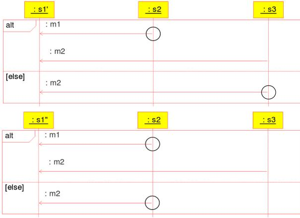
**Figure 4: UML sequence diagram for  $s'_1, s_2,$  and  $s_3$  (on the top: circles underline the race condition between  $s_2$  and  $s_3$ , both of them may send a message at the same time) and for  $s''_1, s_2,$  and  $s_3$  (on the bottom: there is no race condition).**
