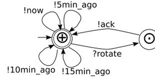
**Figure 2: The Surveillance protocol: a modified Sensor, which also supplies data collected fifteen minutes ago.**
