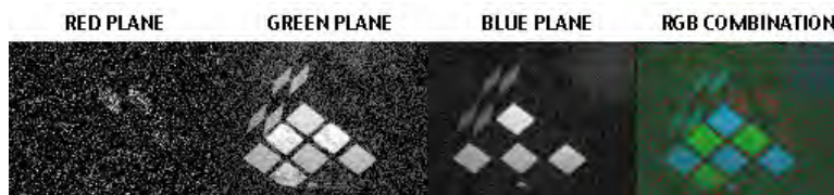
Figure 4. Color plane and RGB combination reconstructions from filtered diode voltage signals under short-wavelength illumination at 128 \times 96 pixel resolution. Produced from a high measurement number ( > 10 \times Nyquist) this non-compressed result shows fluorescence in the green plane and fainter fluorescence in the red, blue is simply the reflection plane.
