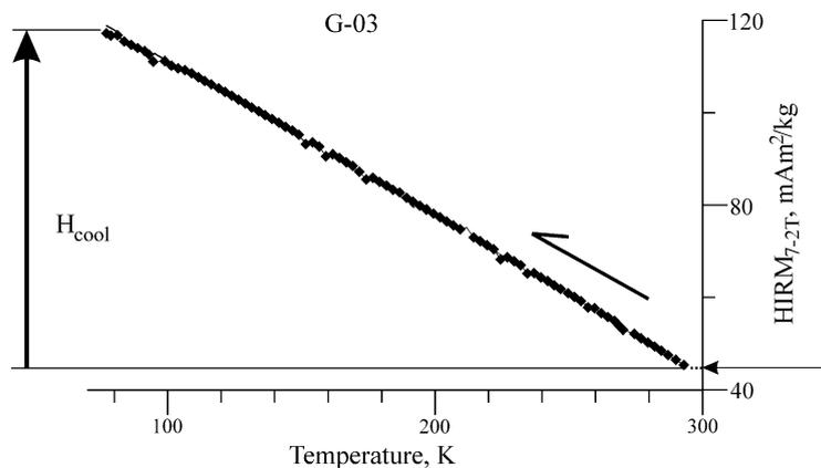
Fig. 6. Low-temperature behaviour of the mass-specific  $HIRM_{7-2 T}$ , illustrating the typical linear rise for goethites, and the new parameter,  $H_{cool}$ . The arrow marks the RT value of the  $HIRM_{7-2 T}$ .
