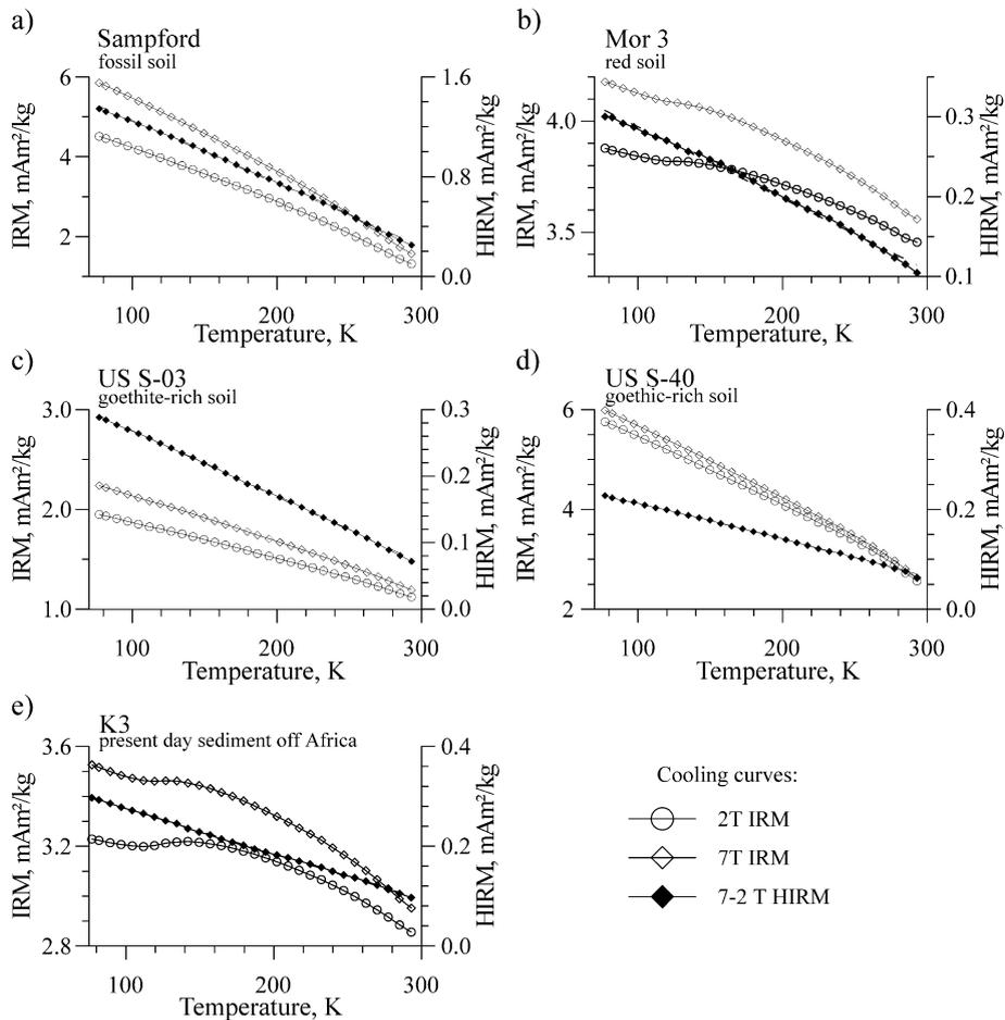
Fig. 10. 2 and 7 T RT IRM cooling curves, from 293 down to 77 K and  $\text{HIRM}_{7-2\text{T}}$  for a range of red and yellow soils. The Verwey transition in magnetite, at around 120 K, is clearly evident in the IRM curves but is removed in the HIRM curve for the samples shown in (b) and (e).
