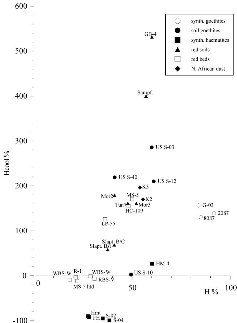
Fig. 11. Biplot of H% versus  $H_{cool}$ % for all synthetic and natural samples. The strong viscosity (at 293 K) in the finest synthetic haematite, HM-4, made it difficult to calculate its H% value.
