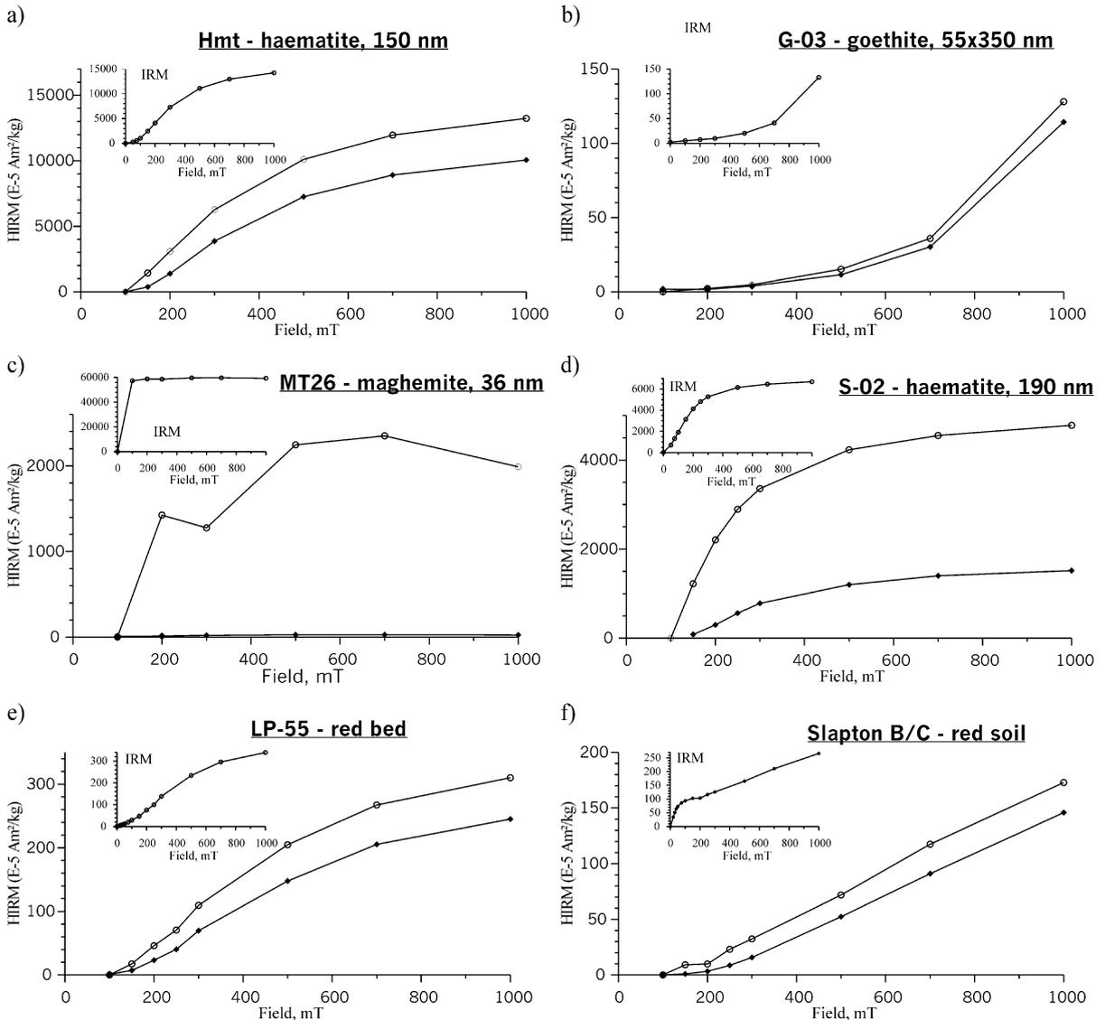
Fig. 4. IRM acquisition curves (shown as inserts) and the stepwise acquisition (open circles) and af demagnetisation (at 100 mT, closed circles) of  $IRM_{>0.1 T}$  for: synthetic haematites (a, d), goethite (b), maghemite (c) and British red bed (e) and red soil (f).
