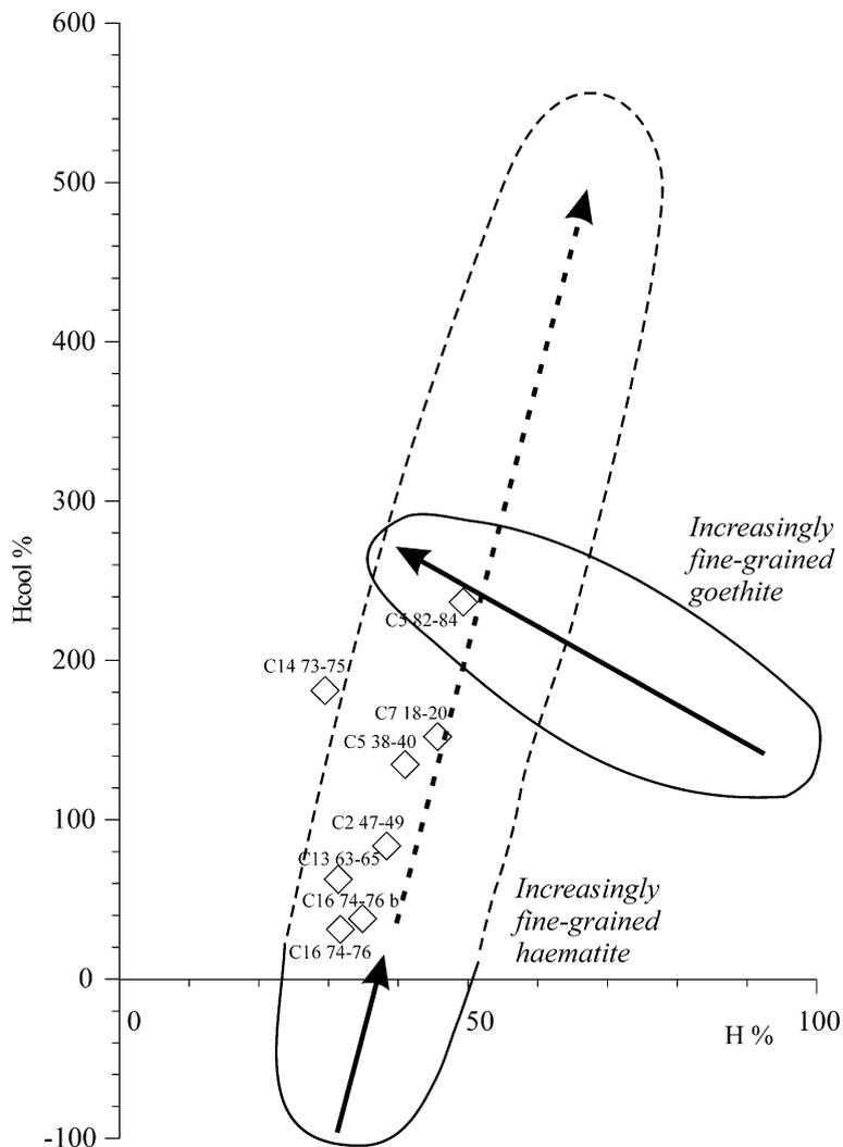
Fig. 12. Biplot of H% versus  $H_{\text{cool}}\%$ , showing envelopes of values for synthetic and natural sample mineralogies, and Australian Holocene fen sediments added. The dashed line indicates the suggested decreasing trend in haematite grain size, towards the SP boundary.
