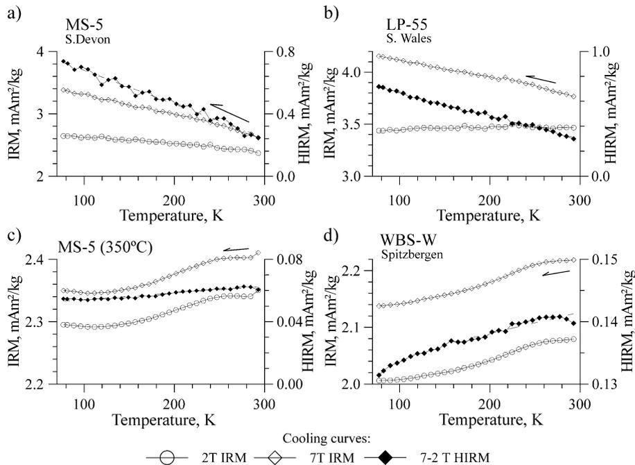
Fig. 9. 2 and 7 T RT IRM cooling curves and  $\text{HIRM}_{7-2\text{ T}}$  for red beds from Britain and Spitzbergen.
