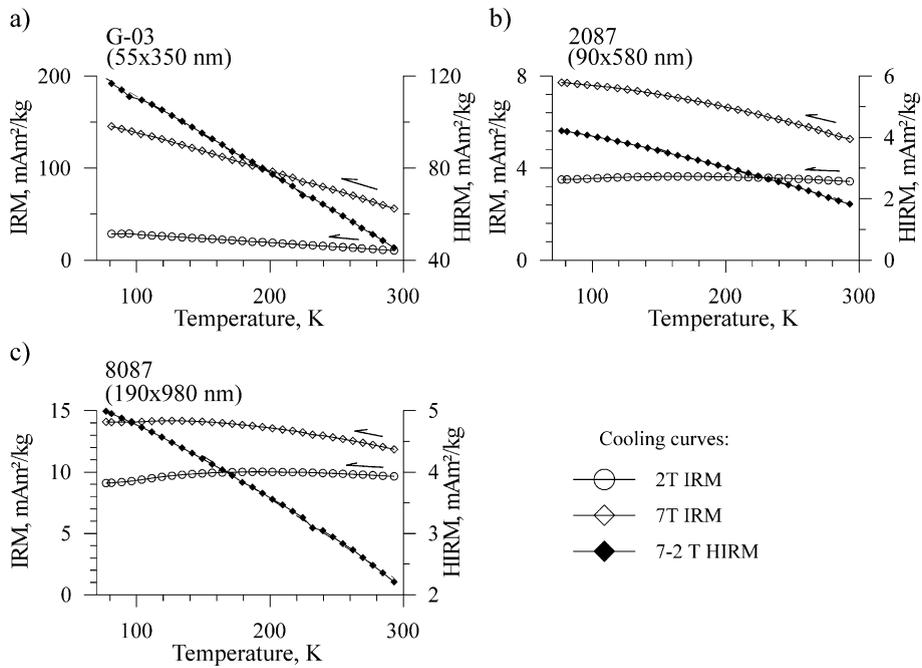
Fig. 7. 2 and 7 T RT IRM cooling curves, from 293 down to 77 K and the calculated  $HIRM_{7-2 T}$  for synthetic goethites. Each sample was subjected to the following sequence of treatments: 2 T at RT; cooling to 77 K; warming to RT; 7 T at RT; cooling to 77 K; warming to RT. Only every third measurement point, at 7.5 K intervals, is shown, for clarity.
