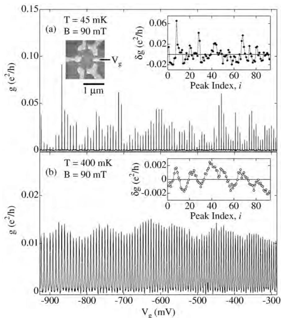
FIG. 1. Coulomb blockade peaks in conductance  $g$  as a function of gate voltage  $V_g$  at (a) 45 mK and (b) 400 mK from device 1. Insets: SEM micrograph of device 1. Peak height fluctuations  $\delta g_i$  extracted from these data sets.
