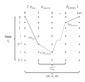
Fig. 3. Trellis diagram for the parity check weight calculation of a punctured RSC code (k=1).
