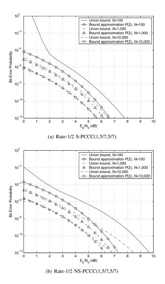
Fig. 4. Exact union bounds and their approximation for punctured rate-1/2 systematic (S-PCCC) and nonsystematic (NS-PCCC) turbo codes employing an interleaver of size 100, 1000 or 10000.
