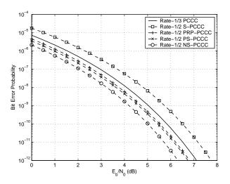
Fig. 5. Bound approximations for the rate-1/3 PCCC(1,5/7,5/7) and various rate-1/2 child configurations. The size of the interleaver is 10,000.
