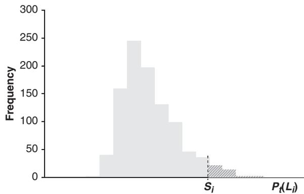
**Fig. 5.** Histogram of simulated probabilities  $P_t(L_i)$  of water shortages of severity  $L_i$ , being imposed in year  $t$ .
