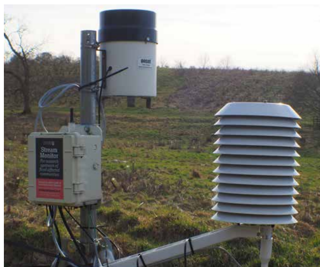
Relative humidity sensor at the Bessy conifer evaporation plot.
