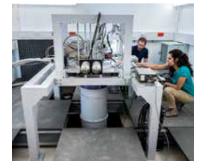
Studying graphene devices at millikelvin temperatures
