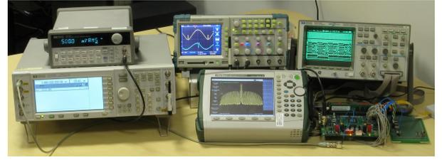
Fig. 12. *MCBC* testbed: IQ modulator with Tx antenna (left), oscilloscope showing the Ultraspherical signal (top center), spectrum analyzer showing its spectrum (bottom center), logic analyzer showing synchronized strobes in its upper part and the random contention signals in its lower part (top right), FPGA platform and independent quartz oscillators board (bottom right).
