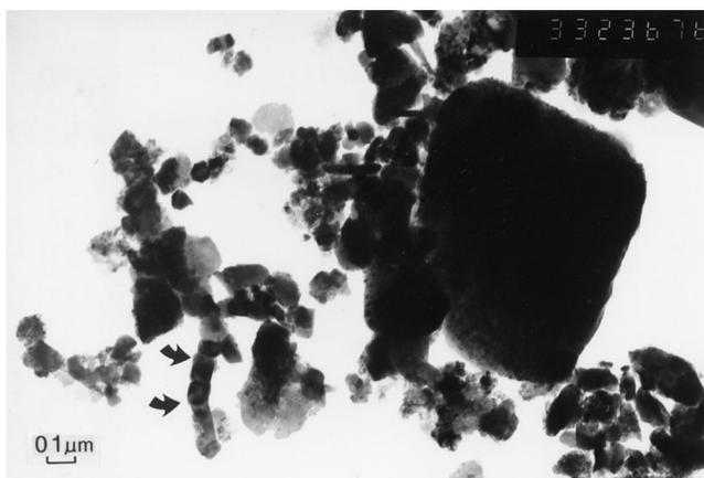
Fig. 6. Transmission electron micrograph of unidimensional, ultrafine ferrimagnets from palaeosol  $S_1$ ; these crystals are formed intracellularly by magnetotactic bacteria. Such biogenic grains constitute  $< 1\%$  of the ultrafine magnetic fraction.
