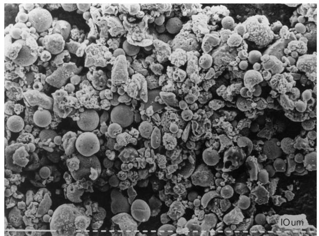
Fig. 1. Scanning electron micrograph of magnetic spherules (pollutant particles), deposited on a surface soil sample (from Maher, 1998).
