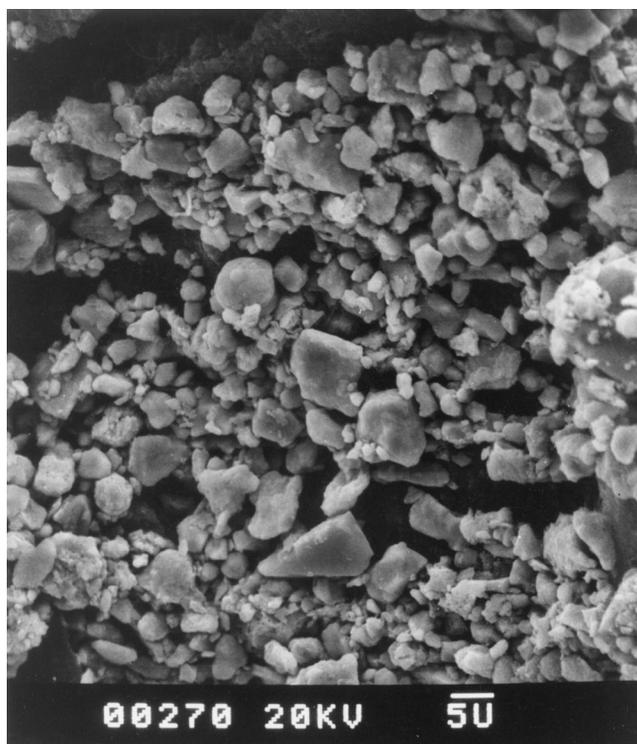
Fig. 7. Scanning electron micrograph of the 'coarse-grained' magnetic fraction from palaeosol  $S_1$ . From X-ray diffraction, these windblown detrital grains are a mixture of magnetite, titanomagnetite and haematite.
