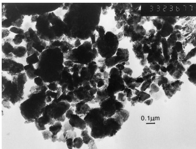
Fig. 5. Transmission electron micrograph of ultrafine ferrimagnets from palaeosol  $S_1$ , Chinese Loess Plateau. Note the very variable grain size ( $\sim 1$ – $100$  nm), indicating *extracellular* precipitation, and clustering of the finest particles around larger grains. Such grains make up  $\sim 99\%$  of the ultrafine magnetic fraction and contribute  $\sim 90\%$  of the magnetic susceptibility signal (Maher and Thompson, 1992).
