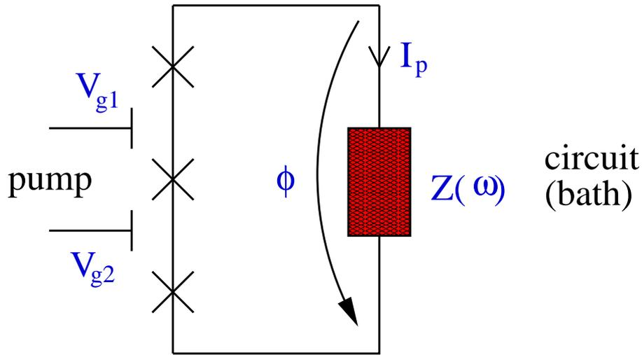
**Circuit:** Total phase difference across pump fluctuates
