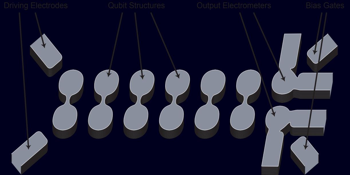
We need to integrate the qubits to make quantum gates, with controlled qubit-qubit interactions, state initialisation, control during processing, and readout.
