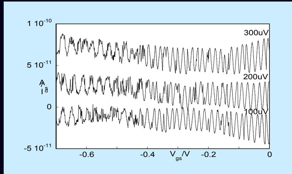
A gated double quantum dot made from a silicon - silicon germanium heterostructure. When the electronic structure changes from one dot to two in series, the noise is reduced.
