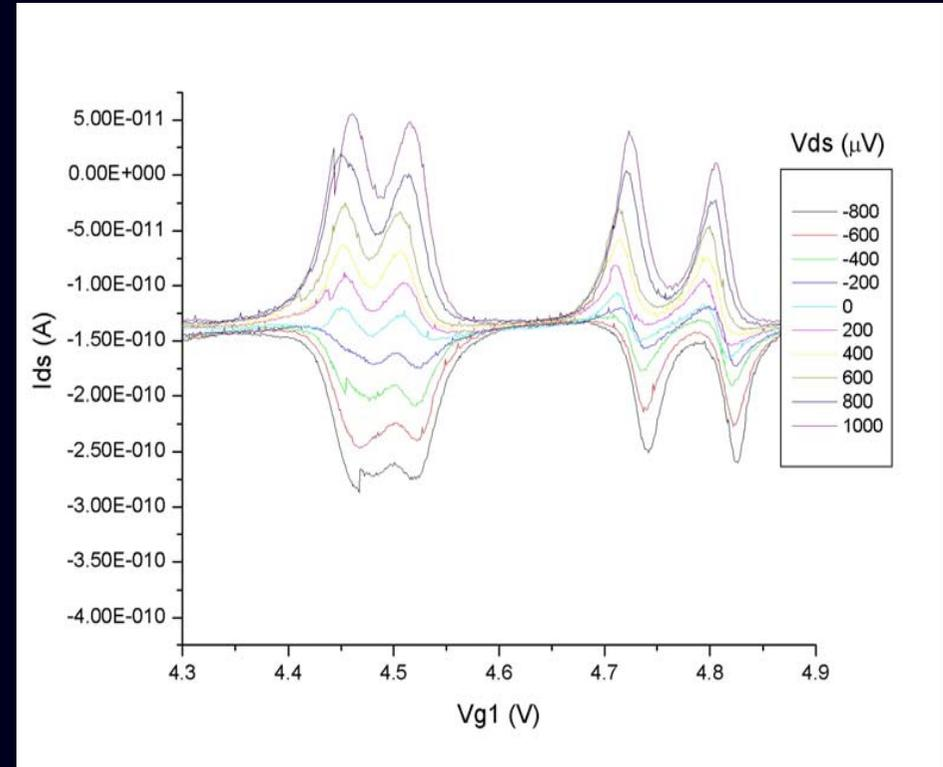
With no source-drain bias, at 20mK, currents are observed due to electron tunnelling driven by 4.2K black-body radiation
