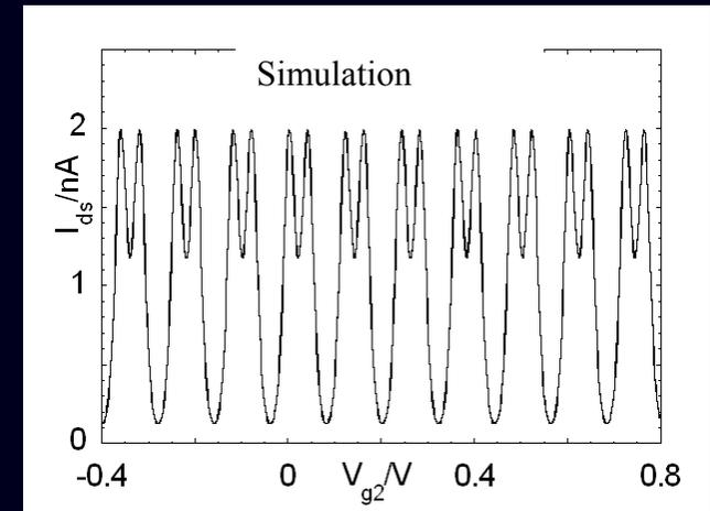
Effective dot size is 30nm - peak splitting is seen at 4.2K instead of previously at 50mK
