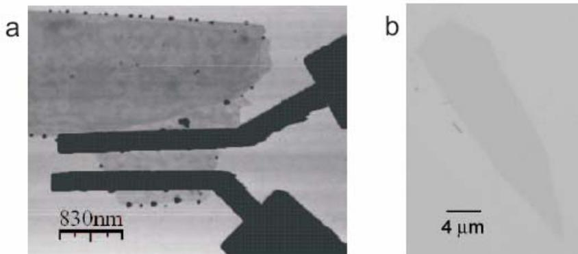
**Fig. 2.** (a) Atomic force microscopy image of a single-layer graphene Josephson junction used in our experiments. The electrodes consist of a Ti/Al bilayer, with the Titanium in contact with graphene. (b) Large graphene layer deposited on top of a Si/SiO<sub>2</sub> substrate by controlled exfoliation of a single graphite crystal. graphpe
