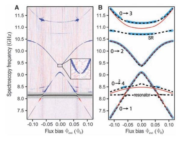
Lines allow first finding and then verifying the model parameters
