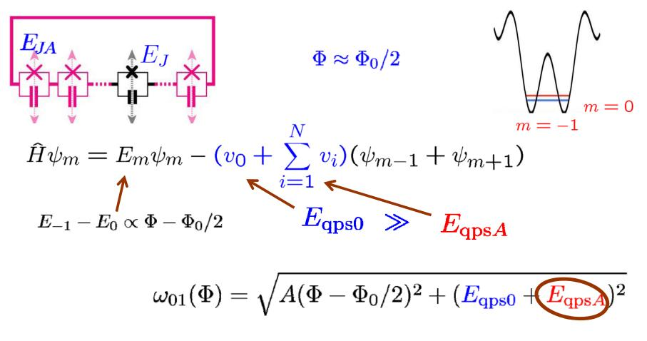
Transition frequency is most sensitive to a QPS in array at  $\Phi \approx \Phi_0/2$
