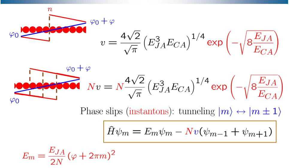
Weak dependence of the ground state energy on phase difference at  $Nv \gg E_J/N$
