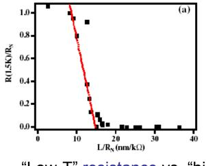
"Low-T" resistance vs. "high-T" resistivity
