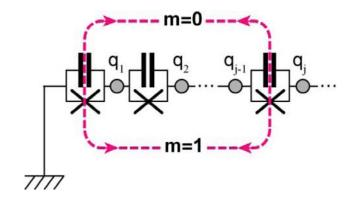
Cycling a phase slip brings in a phase factor  $\boldsymbol{n}$  $p_n = \sum_{j=1}^{n} q_j$  charge = A-C phase
