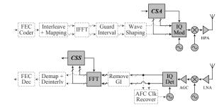
Fig. 4. PHY transceiver. During the CW, only the shaded blocks are active, the dashed blocks are skipped and disabled. During data exchange, the CSA and CSS blocks are skipped and disabled while the other blocks are active.
