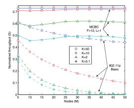
Fig. 19.  $\it MCBC$  without fading protection ( $\it L=1$ ) and IEEE 802.11p in basic access mode.
