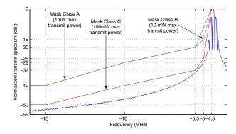
Fig. 7. Worst case transmit spectrum:  $\Phi = 4$ ,  $N_{CP} = 32$  and active *MCBC* subcarrier index -28. Mask Class D is not shown as it is meant only for very high transmit powers (max 760 mW).
