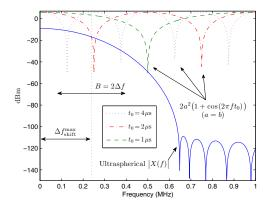
Fig. 8. FFT response of Ultraspherical burst and worst case combined time shift component from two simultaneous transmissions ( $t_0$  is the time shift).
