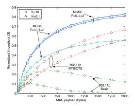
Fig. 21. Normalized throughput vs. MAC payload for deep  $(K\!=\!0.1)$  and low fading  $(K\!=\!10)$  and  $M\!=\!25$  active nodes.
