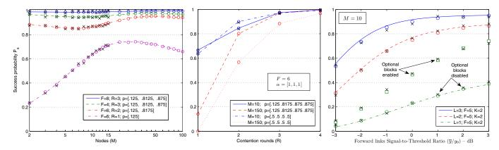
Fig. 18. MCBC success probability  $P_s$ ; Analysis vs. measurements vs. simulations: variable number of nodes in ideal channel (left), variable number of rounds in ideal channel (center) and variable fading (right). Lines represent theoretical analysis, circle markers represent software simulations and crosshair markers show hardware measurements. The square markers (right) represent results when the optional blocks of the algorithm (see Fig. 2) are enabled.
