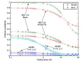
Fig. 22. Collision probability vs. fading severity, from deep (low K) to no fading (high K), for 5 and 50 active nodes.
