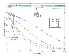
Fig. 20. MCBC with fading protection (L=3) and IEEE 802.11p with RTS/CTS enabled.
