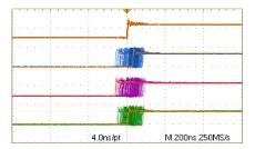
Fig. 17. Persistent oscilloscope showing synchronized slot strobes (100 ns sync accuracy) of 100 kHz derived from 100 ppm independent oscillators. The sync strobe (top) is 1 pps derived from a 10 MHz 100 ppm oscillator.
