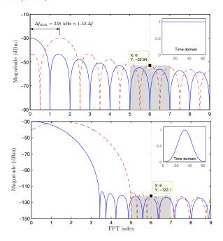
Fig. 6. Frequency response of the rectangular window (left) and Ultraspherical window (right). Full lines represent the ideal response for synchronized center frequencies between the transmitters and the receiver while dashed lines represent the actual response due to frequency shift. The shaded boxes represent the effective FFT filter bandwidth per subcarrier,  $B=2\Delta f$ .
