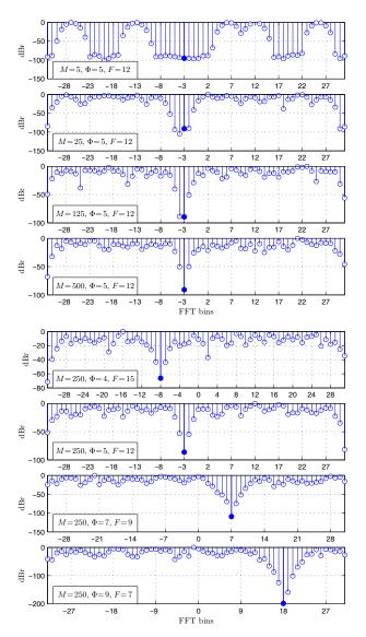
Fig. 9. Normalized response of MCBC bursts spaced in frequency with  $\Phi \Delta f$  for M simultaneously transmitting nodes, random time shift in the range  $[0,4]~\mu s$ , random frequency shift in the range [-238,238] kHz and  $-174~{\rm dBm/Hz}$  receiver noise. The 6<sup>th</sup> MCBC subcarrier index (full marker) was intentionally avoided by all nodes to validate the burst detection mechanism. Only the numbered FFT bins are read by MCBC during contention.
