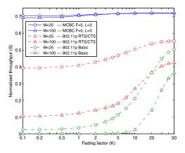
Fig. 23. Normalized throughput vs. fading severity, from deep (low K) to no fading (high K), for 25 and 100 active nodes.
