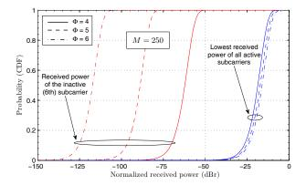
Fig. 10. Received power CDF of the inactive (6<sup>th</sup>) *MCBC* subcarrier and of the highest attenuated active *MCBC* subcarrier.
