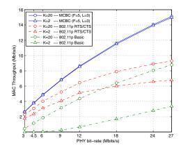
Fig. 24. Throughput for all PHY bit-rates in low (K=20) and moderate fading (K=2) channels for M=25 nodes.
