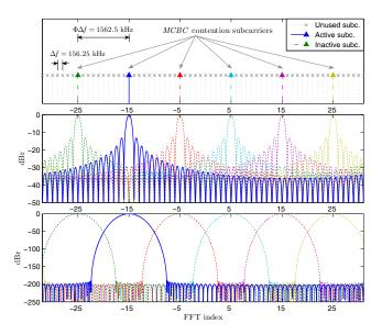
Fig. 5. F=6 contention subcarriers spaced with  $\Phi=10$  times the normal OFDM subcarrier spacing,  $\Delta f=156.25$  kHz [1]. Symbolic spectrum (top), normalized spectrum using a rectangular window (middle) and Ultrashperical window (bottom).
