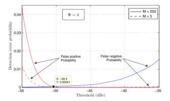
Fig. 11. Detection error probability versus detection threshold.
