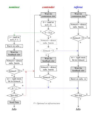
Fig. 2. Contention algorithm running in a node. The node enters contention from Idle as *contender* if it has data to send. In an adhoc network, if it does not have data to send, the node may choose to remain idle or start as *referee*. In an infrastructure network, the AP is the dedicated and only referee, following the same algorithm, and the blue dashed transitions do not exist. Dashed lines represent transitions between *contender*, *nominee* and *referee* states.
