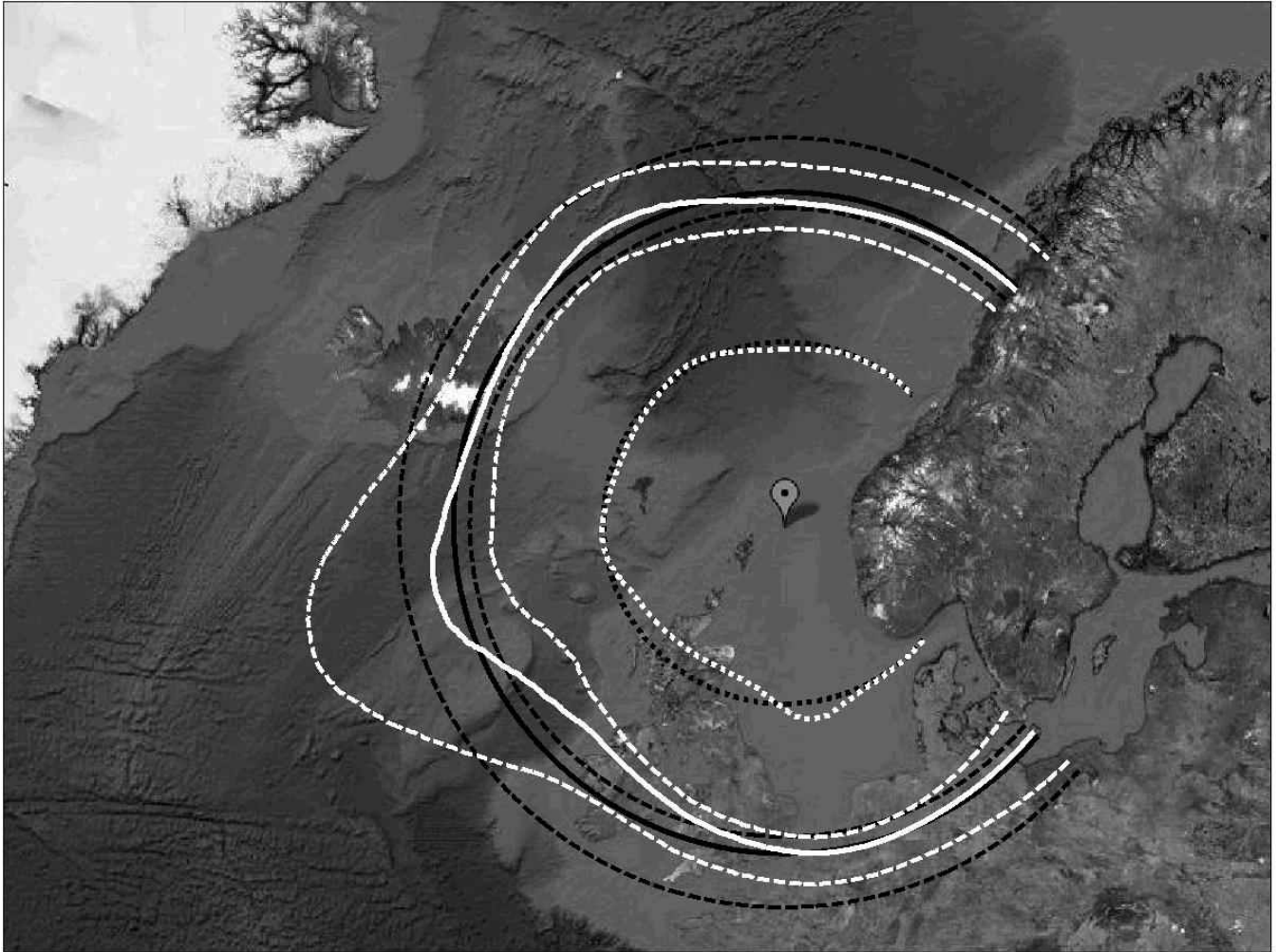
Figure 6: Return values of storm peak H_S (inner circle) and associated conditional values of T_P (outer circle). Inner dashed lines (on common scale): storm peak H_S with non-exceedance probability 0.99 (in 34 years), with (white) and without (black) directional effects. Outer solid lines (on common scale): median associated T_P with (white) and without (black) directional effects; outer dashed lines give corresponding 2.5% and 97.5% percentile values for associated T_P . Design values are withheld for reasons of confidentiality.
